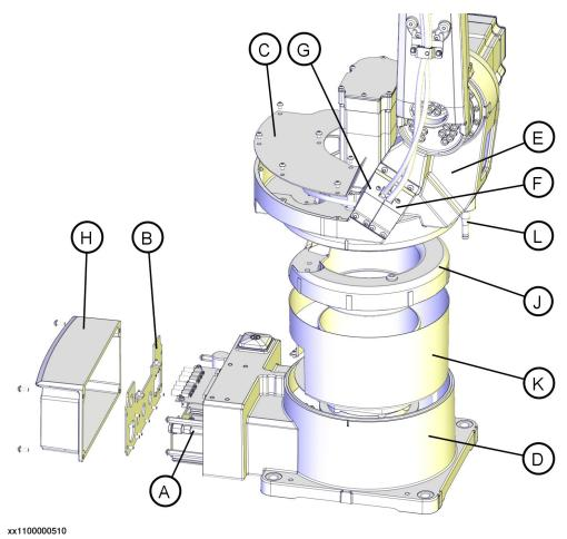
1.7 Spare parts - cable harness, brake release and SMB
